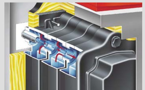
Increased boiler life and efficiency with return injector (with Vitotronic controls)
